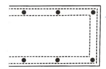
**Grommet and Fasteners** – Spur-toothed, rolled-rim grommets are recommended. Washer-type grommets have a tendency to slide on the fabric and pull out. Insert grommets every one to two feet along edges of the banner and mount between stitch lines of the hem, leaving at least 1/8" inch (1/3 centimeter) from the grommet edges to the stitch line.
